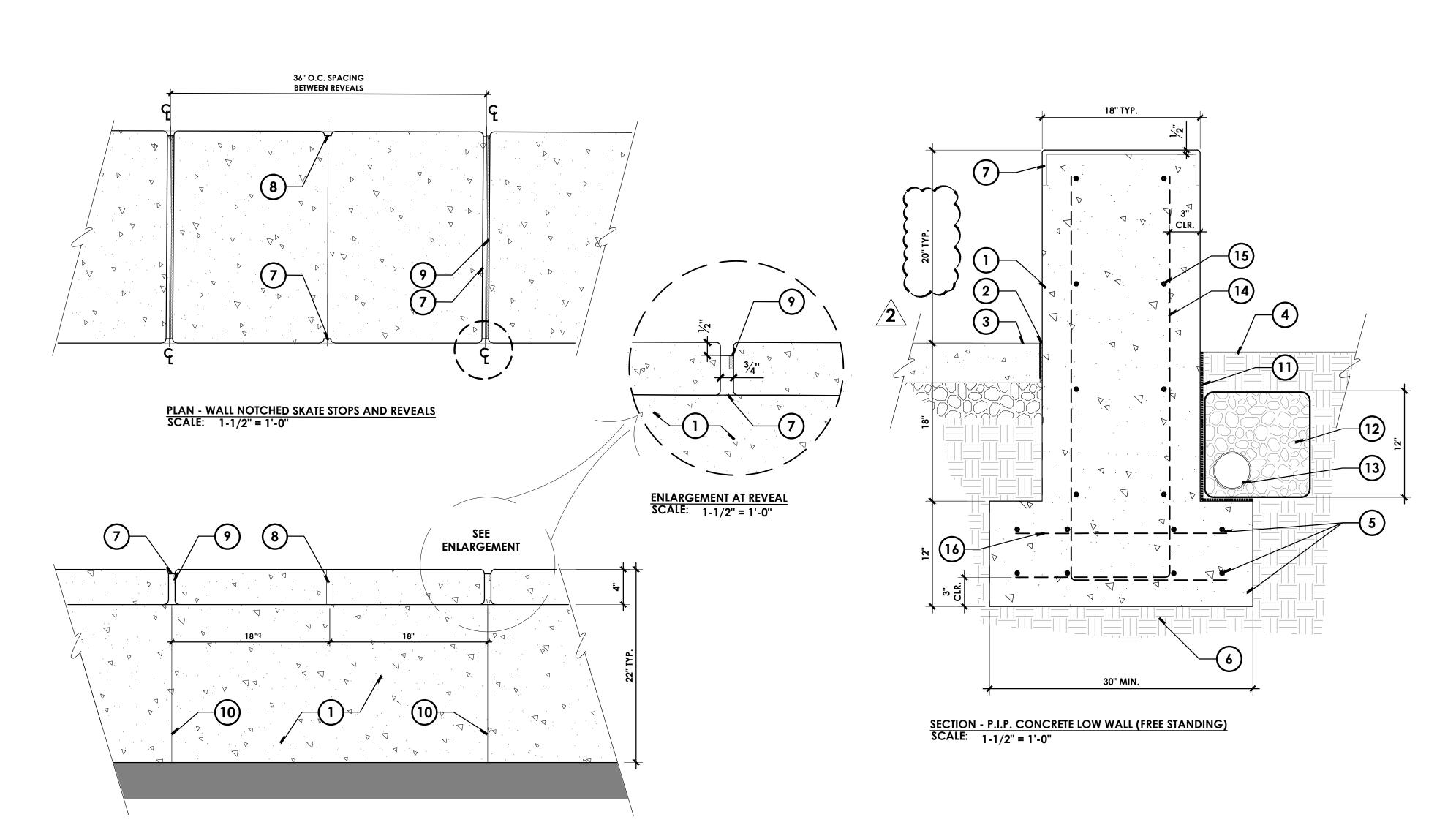
ELEVATION - WALL NOTCHED SKATE STOPS AND REVEALS SCALE: 1-1/2" = 1'-0"
