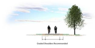
CLASS I - Multi-Use Path Provides a completely separated right-of-way for exclusive use of bicycles and pedestrians with crossflow minimized.
