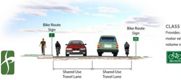
CLASS III - Bike Route Provides a shared use with pedestrians or motor vehicle traffic, typically on lower volume roadways.
