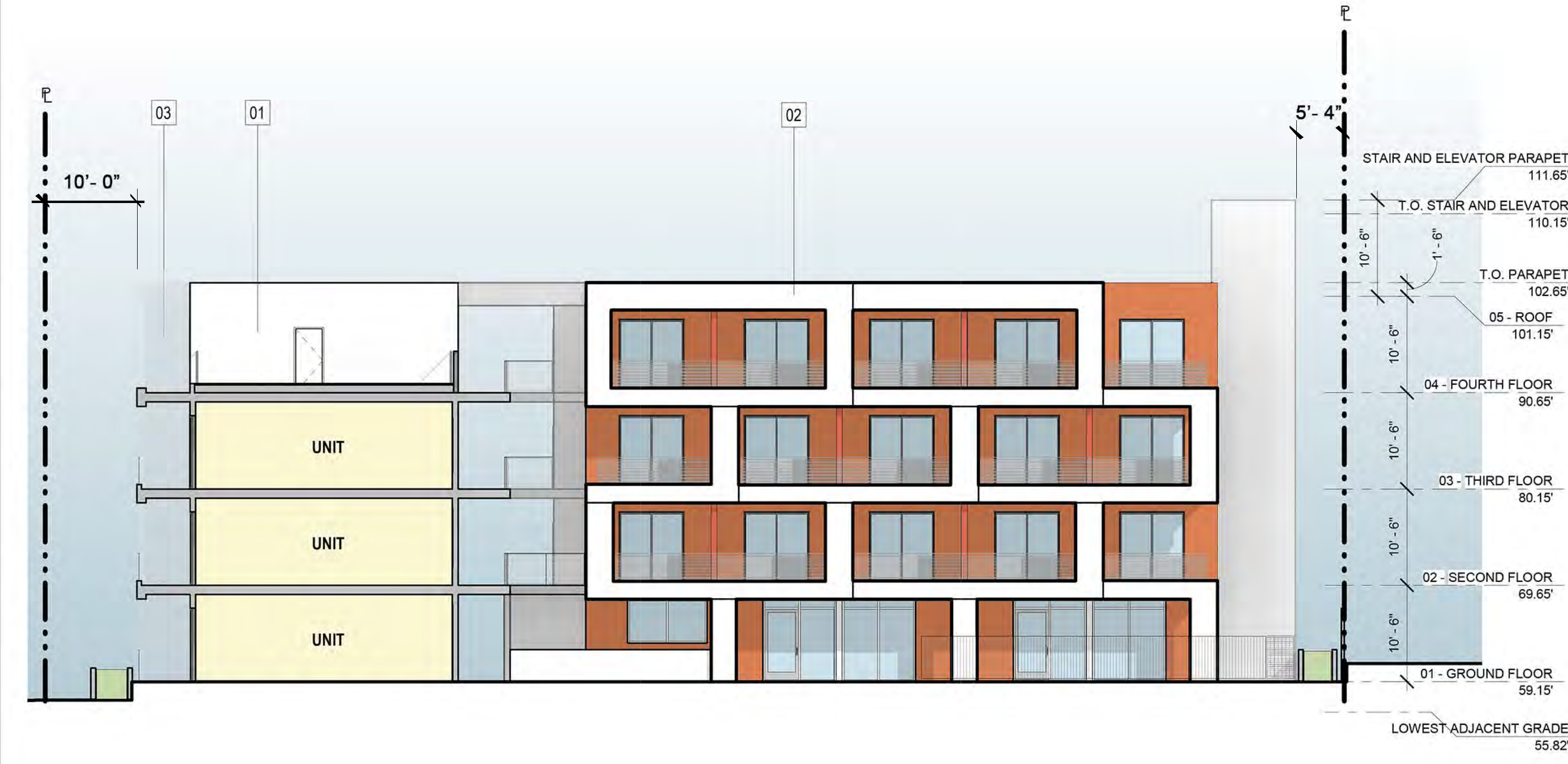
COURTYARD ELEVATION - NORTH SCALE: 3/32" = 1'- 0"
