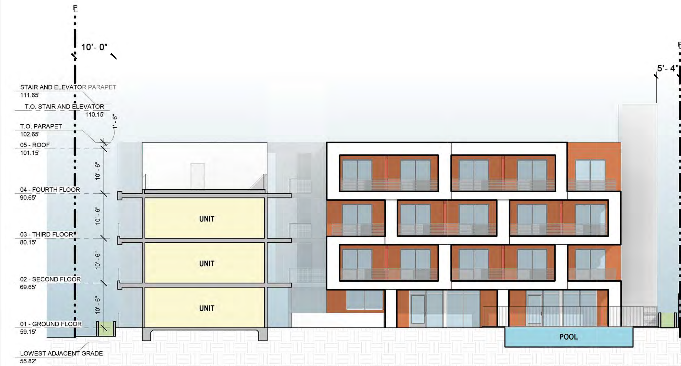
ELEVATION / CROSS SECTION THROUGH COURTYARD - NORTH SCALE: 3/32" = 1'- 0"
