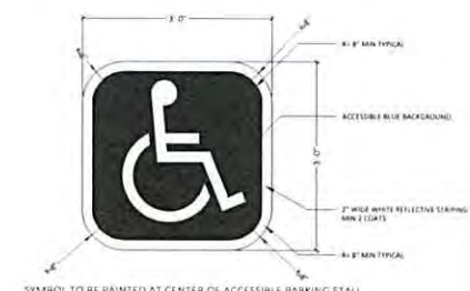
2 ACCESSIBLE PARKING STALL FLOOR SIGN SCALE: 1/4" = 1'-0"
